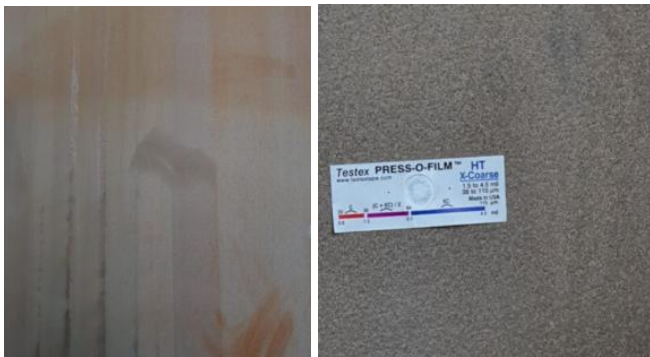
Figure 6 Test plate surface post-Robotic WAB (single nozzle) (Left: Normal view. Right: Magnified view)
