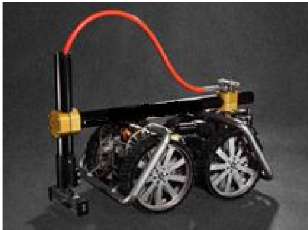
Figure 2 WAB robot with a single-nozzle system equipped with carrier and swing arm
