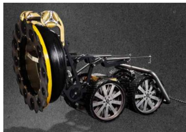
Figure 1 UHP WJ robot with vacuum dome
