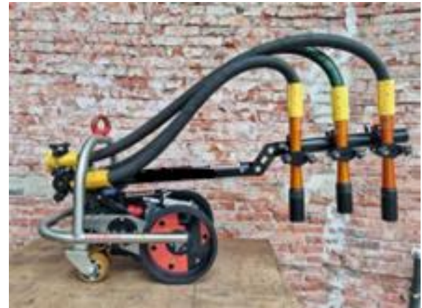
Figure 3 WAB robot with a three-nozzle system equipped with a carrier and swing arm
