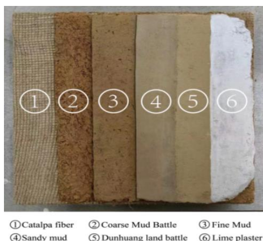
Figure 4: Wall making process
