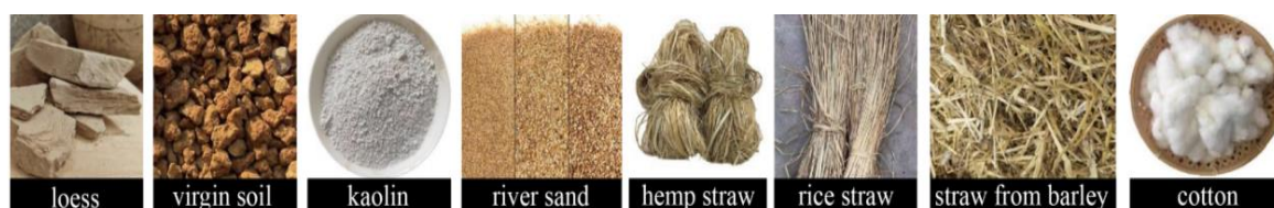
Figure 3: Materials for making the base layer
