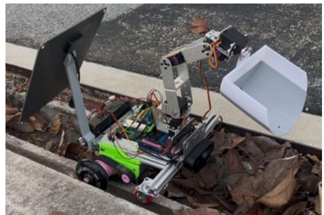
Figure 5 Assembled autonomous drain-cleaning robot prototype
