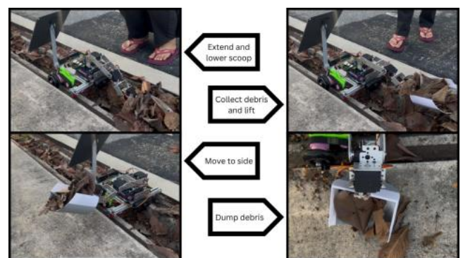
Figure 6 Sequence of autonomous debris collection during field testing in a residential concrete drain
