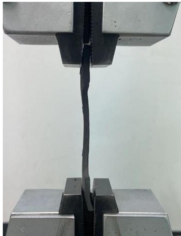
Figure 7 Uneven sample clipped by the universal tensile machine
