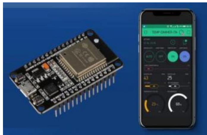
Figure 1: ESP32 and Blynk Application
