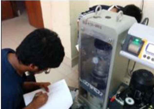
Figure 6 Compressive strength testing of concrete specimen
