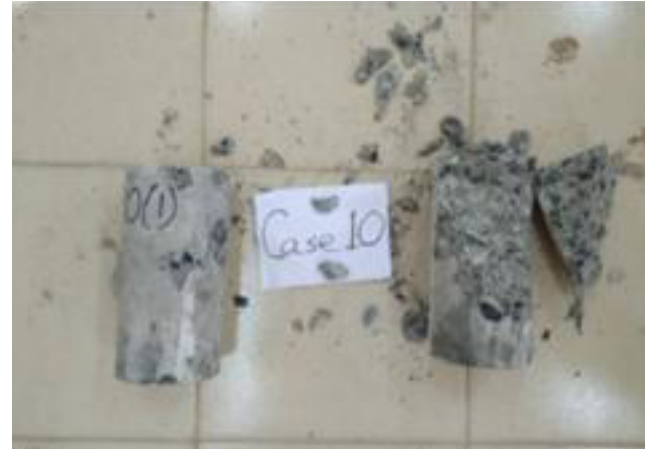
Figure 6 Compressive strength testing of concrete specimen
