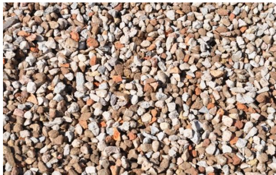
a. Recycled brick aggregates
