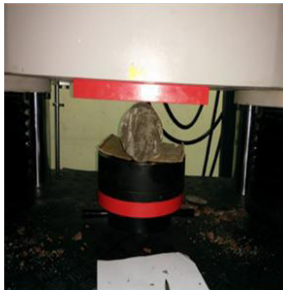
Figure 2 Split tensile strength test by UTM
