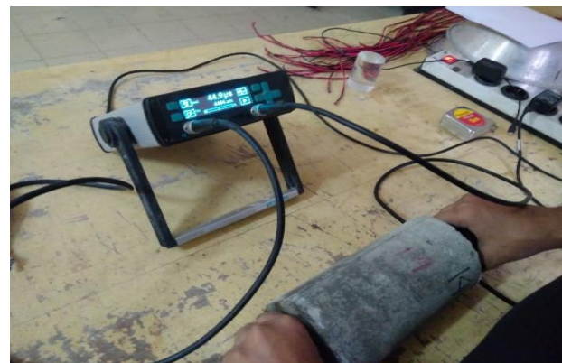
Figure 4 UPV test of concrete specimen
